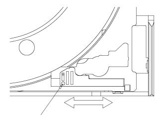
3. First hang a disc on a disc holder in an upper and rear side of a tray, and then put the disc on disc holders in a down side of the tray.
